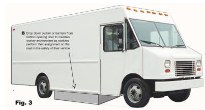
The bottom opening can be any typ of door including waterproof cloth covering, a hinged or unhinged door or multiple doors or roll up door and similar.
