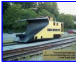
Unlike this 100 year old train, modern railroad snow removal trains employ snow blowers that run at relatively high speeds.
