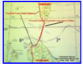
The Sakhalin-Hokkaido Long Tunnel would be 42km long and could be constructed in 9 years, at the cost of approximately 4.2 Billion (thousand million) U.S. Dollars
